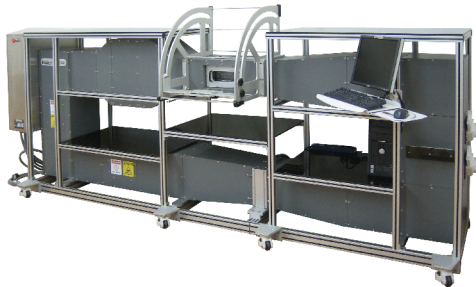
Fig. C: FDK Original Wind Tunnel
