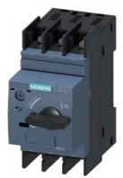
Circuit breaker size S00 for motor protection, CLASS 10 A-release 1.4...2 A N-release 26 A ring cable lug connection Standard switching capacity
