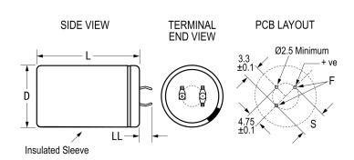
General Information Series ALC80 Dielectric Aluminum Electrolytic Description Snap-In, Aluminum Electrolytic RoHS Lead 3 Pin Short AEC-Q200 No Halogen Free Yes Component Weight 65 g Notes Dimensions D And L Include Sleeving. Shelf Life 156 Weeks
