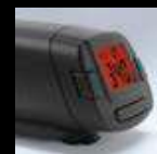
Visual warning: too hot = red
