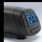
Visual warning: too cold = blue
