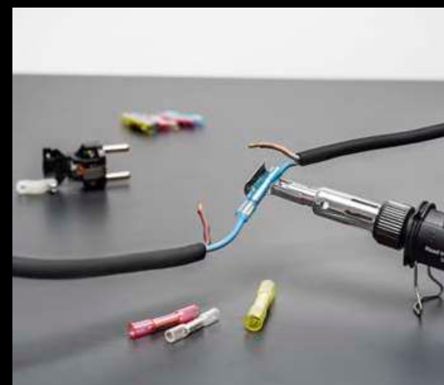
Create an even seal on solder sleeves
