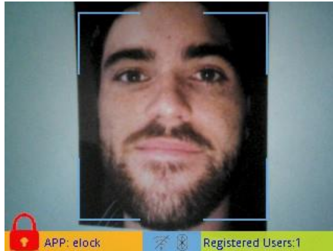
Figure 14: Printed Picture SpooF Attack
