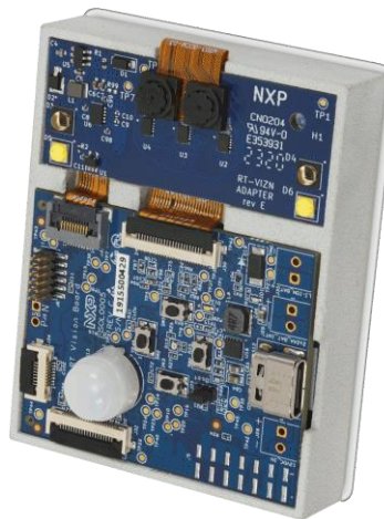
Figure 2: Dual Camera Adapter Kit Configuration
