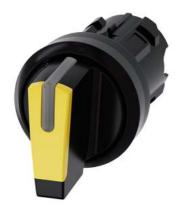
Selector switch, illuminable, 22 mm, round, plastic, yellow, selector switch, short, 3 switch positions I-O<II, left latching, right momentary contact type, actuating angle  $2x45^{\circ}$ , 10:30h/12h/13:30h Z=50-unit packaging
