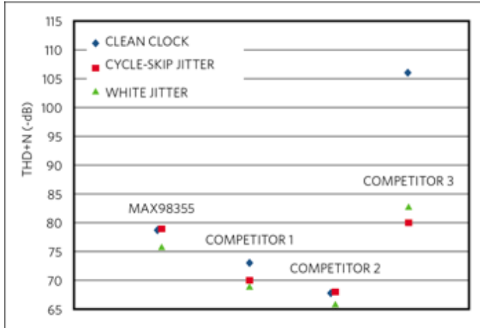
Figure 10. 1kHz THD+N performance degradation with clock jitter.
