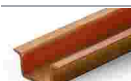
Item no.: 210-198 Copper carrier rail; 35 x 15 mm; 2.3 mm thick; 2 m long; unslotted; according to EN 60715; copper-colored
