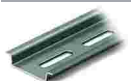
Item no.: 210-504 Steel carrier rail; 35 x 7.5 mm; 1 mm thick; 2 m long; slotted; galvanized; according to EN 60715; silver-colored
