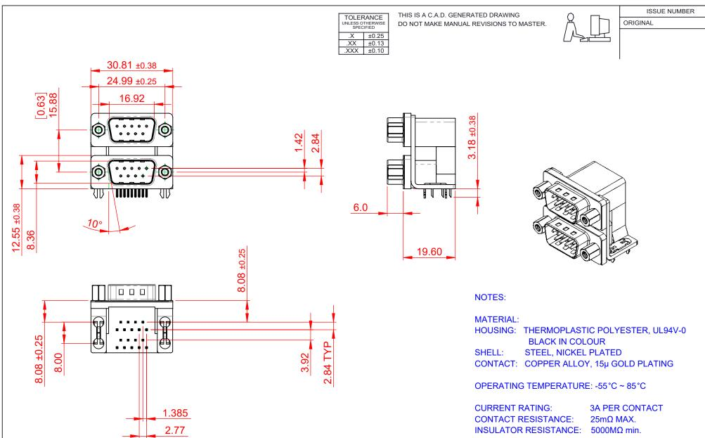
DIELECTRIC WITHSTANDING VOLTAGE: 1000V AC rms (1)
