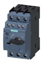
Circuit breaker size S0 for motor protection, CLASS 10 A-release 1.1...1.6 A N-release 21 A screw terminal Standard switching capacity with transverse auxiliary switches 1 NO+1 NC
