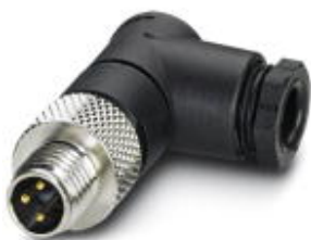
Connector, Universal, 3-position, Plug angled M8, A-coded, Solder connection, knurl material: Nickel-plated brass, external cable diameter 3.5 mm ... 5 mm
