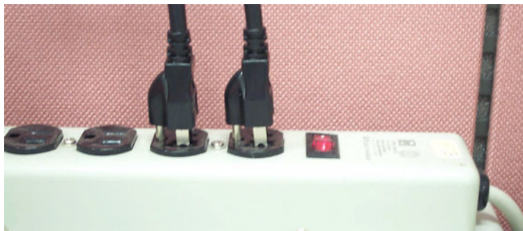
Figure 3.8 Power cord plugs should have same orientation in socket/ 插座上电源线方向相同 / 插座上的電源線方向應相同
