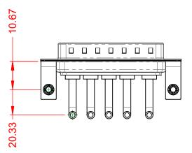
20A (CURRENT) POWER/CO-AX CONTACT RATING: (IF PRESENT) SIGNAL CONTACT CURRENT RATING: 5A PER CONTACT SIGNAL CONTACT RESISTANCE:  $10m\Omega$  MAX. **INSULATOR RESISTANCE:**
