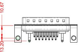
10A (CURRENT) POWER/CO-AX CONTACT RATING: (IF PRESENT) SIGNAL CONTACT CURRENT RATING: 5A PER CONTACT SIGNAL CONTACT RESISTANCE:  $10m\Omega$  MAX.
