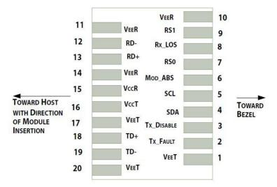
Pin-out of connector Block on Host board
