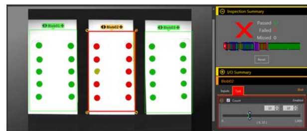
Figure 143. Bad Part—Broken Pill
