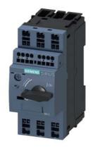
Circuit breaker size S00 for motor protection, CLASS 10 A-release 0.35...0.5 A N-release 6.5 A Spring-type terminal Standard switching capacity with transverse auxiliary switches 1 NO+1 NC
