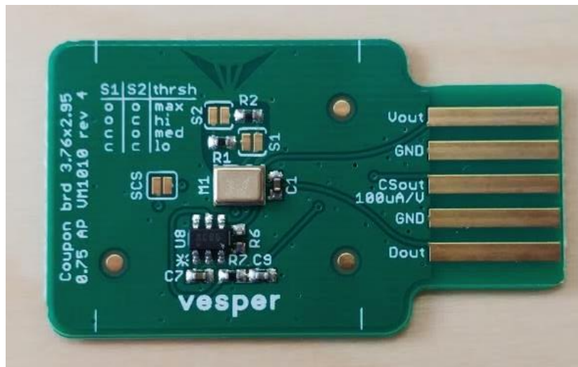
Figure 11: Vesper’s VM1010 Zero Power Evaluation Board (VM1010 microphone seen at the center)
