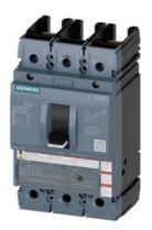
circuit breaker 3VA5 UL frame 250 breaking capacity class H 65kA @ 480V 2-pole, line protection TM210, FTFM, In=90A overload protection Ir=90A fixed short-circuit protection li=10 x In without connection
