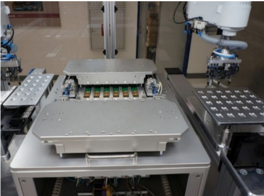
Figure 10: Automatic test equipment for module test
