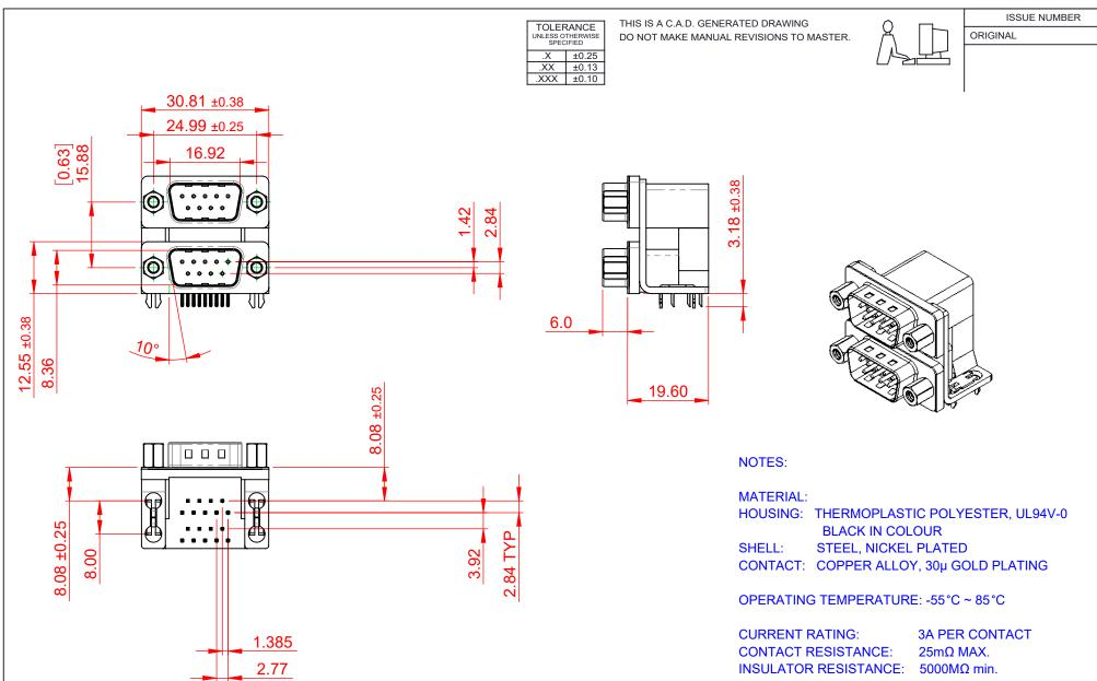
DIELECTRIC WITHSTANDING VOLTAGE: 1000V AC rms (1)
