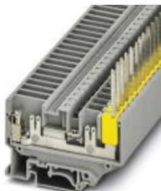
Feed-through terminal block, connection method: Screw connection, TERMI-POINT®, cross section: 0.2 mm 2 - 4 mm 2 , AWG: 24 - 12, width: 6.2 mm, color: gray, mounting: NS 35/7,5, NS 35/15, NS 32
