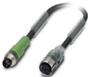
Sensor/actuator cable, 3-position, Variable cable type, Plug straight M8, on Socket straight M12 SPEEDCON, A-coded, with 2 LEDs, cable length: Free input (0.2 ... 40.0 m)
