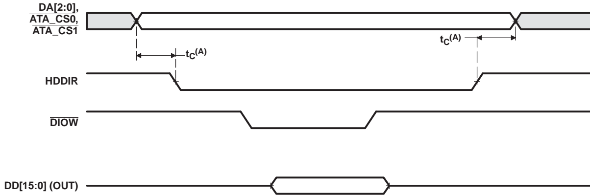
Figure 6-38. ATA/CF HDDIR Taskfile Write/Single PIO Write Timing
