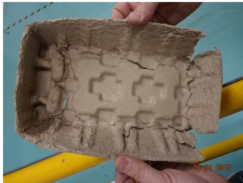
RT1 and C1 pushed in following Front top left drop
