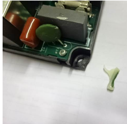
RT1 and C1 pushed in following Front top left drop
