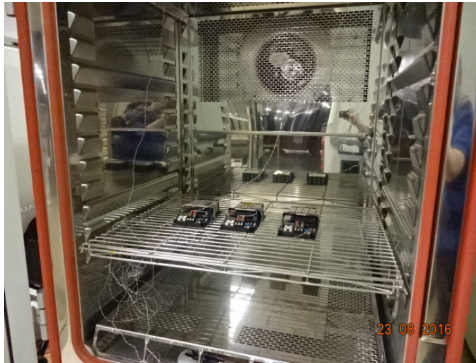
Environmental chamber setup for the non-operational temperature and humidity
