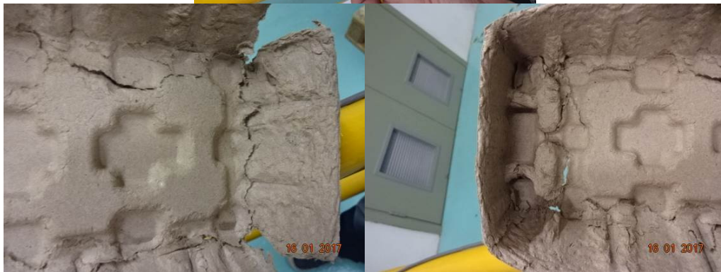
Internal packaging following 17 / 26 freefall impacts
