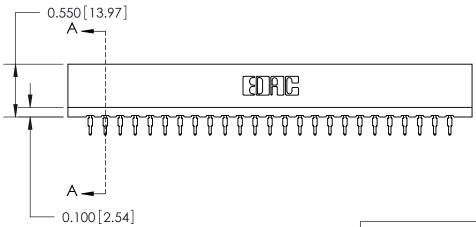
0.420 10.67 Card Slot 0.26 [6.63] 0.23 5.87 Point of Contact 0.550 13.97 0.300 [7.62] SECTION A-A
