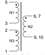
N2 is made of two bifilar windings. Therefore customer has to tie terminals 6+7 and 9+10 on PCB. A general separation of the two windings cannot be guaranteed.
