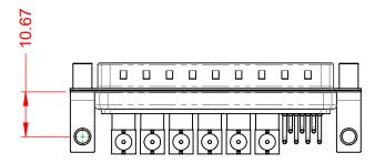
**OPERATING TEMPERATURE:** -55°C ~ 125°C 50Ω (IMPEDANCE) POWER/CO-AX CONTACT RATING: (IF PRESENT) SIGNAL CONTACT CURRENT RATING: 5A PER CONTACT SIGNAL CONTACT RESISTANCE:  $10m\Omega$  MAX. **INSULATOR RESISTANCE:** 5000MΩ min. DIELECTRIC
