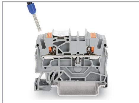
Push-in termination of solid and ferruled conductors
