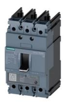
circuit breaker 3VA5 UL frame 125 breaking capacity class M 35kA @ 480 V 3-pole, line protection TM230, FTAM, In=50A overload protection Ir=50A fixed short-circuit protection Ii=5...10 x In UL 489 SB (naval), 50° C without connection
