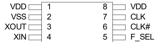
Figure 1. 8-pin TSSOP pinout
