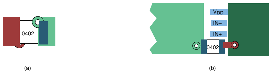
Figure 33. Typical Decoupling Capacitor Layouts
