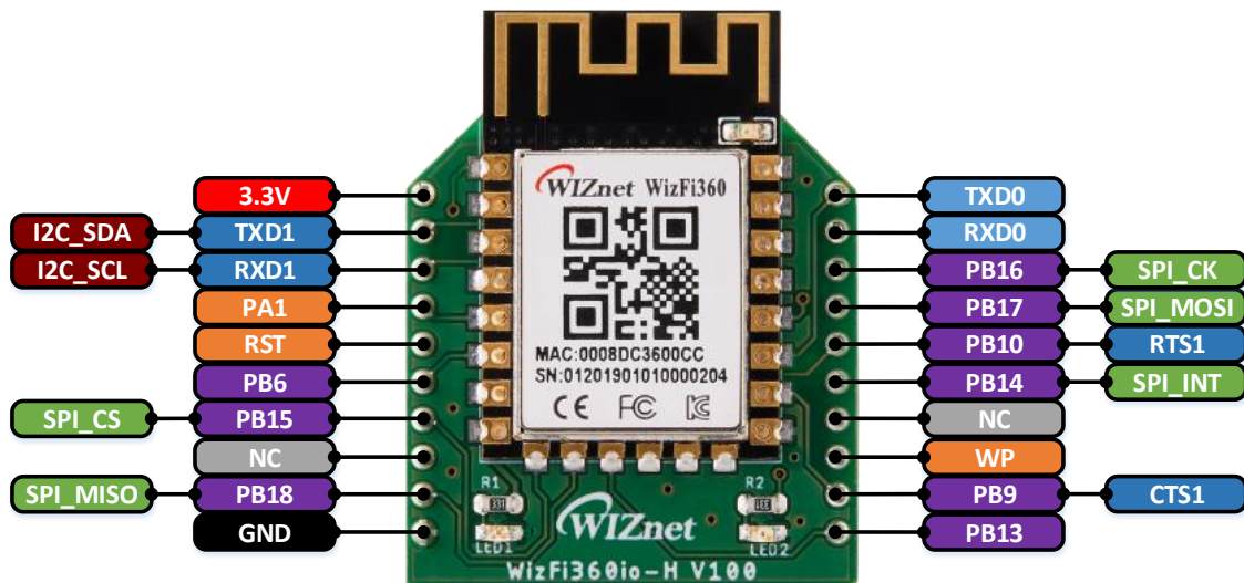
Figure 2. WizFi360io-H Pinout
