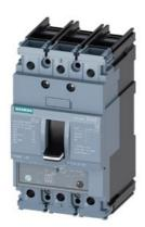
circuit breaker 3VA5 UL frame 125 breaking capacity class S 25kA @ 480 V 3-pole, line protection TM240, ATAM, In=60A overload protection Ir=48A ...60A short-circuit protection Ii=5...10 x In cable connection on both sides
