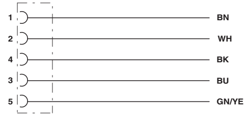
Contact assignment of the M12 sockets
