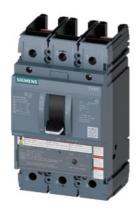
circuit breaker 3VA5 UL frame 250 breaking capacity class C 100kA @ 480V 2-pole, line protection TM230, FTAM, In=90A overload protection Ir=90A fixed short-circuit protection li=5...10 x In without connection
