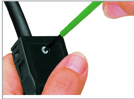
Tighten strain relief screw with screwdriver (2.5 mm blade width).
