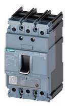
circuit breaker 3VA5 UL frame 125 breaking capacity class H 65kA @ 480 V 3-pole, line protection TM230, FTAM, In=50A overload protection Ir=50A fixed short-circuit protection Ii=5...10 x In UL489 SB (naval), 50 deg. cel. cable connection on both sides
