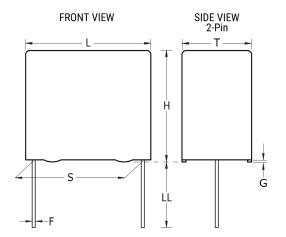
**General Information** Series PFR/F411 Dielectric Film/Foil Polypropylene Style Radial Features Pulse RoHS Yes Lead Wire Leads AEC-Q200 No Component 0.371 g Weight An Operating Temperature Up To +105C Is Allowed Under Certain Conditions. Please Consult Miscellaneous KEMET For Details.
