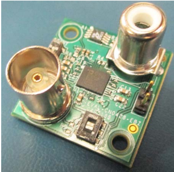
Figure 5. EVAL-CN0428-EBZ Water Sensor Boards
