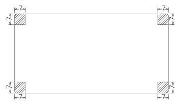
Condition to meet Isolation & Withstand Voltage standard.
