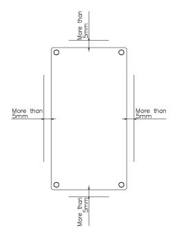
Keep 5mm space from the surfaces and sides of PCB. Especially, 8mm space is necessary from the solder surface. If the space is not enough, the specification of isolation and withstand will not be satisfied.
