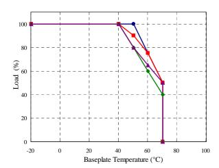
(\*1)Output derating is different depending on the output voltage
