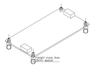
Allowable area by metal pieces is 7mm from each PCB corners. Refer to figure below.
