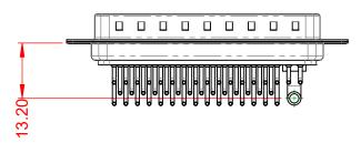
POWER/CO-AX CONTACT RATING:30A (CURRENT)(IF PRESENT)SIGNAL CONTACT CURRENT RATING:5A PER CONTACTSIGNAL CONTACT RESISTANCE:10mΩ MAX.INSULATOR RESISTANCE:5000MΩ min.
