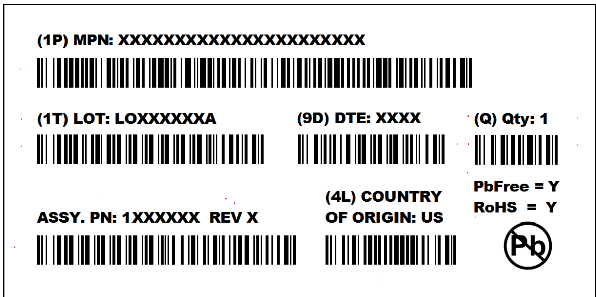
Figure 1. Outer Barcode Label Applied to ESD Bag Packaging
