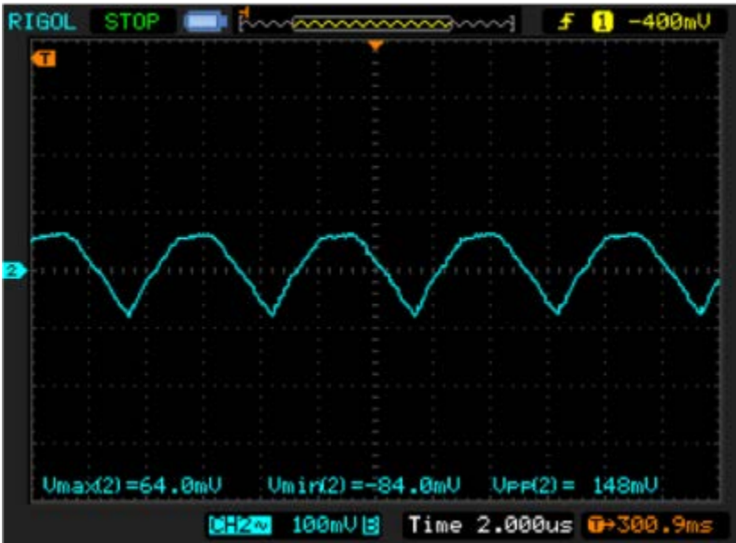
Figure 3. Output ripple at 800mA load, 12V OUT .
