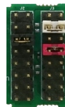
Figure 5: J2 and J3 jumper settings for USB
