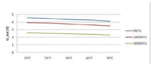
characteristic curve "Voltage ----Temperature
