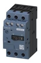
Circuit breaker size S00 for motor protection, CLASS 10 A-release 0.35...0.5 A N-release 6.5 A Screw terminal Standard switching capacity with transverse auxiliary switch 1 NO+1 NC
