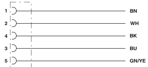
Contact assignment of the M12 sockets
