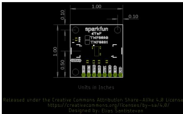
Qwiic dToF Imager - TMF8820/TMF8821 - Board Dimensions
