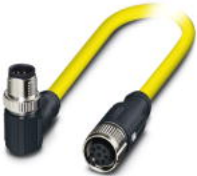
Sensor/actuator cable, 8-position, PVC, yellow, shielded, Plug angled M12 SPEEDCON, A-coded, on Socket straight M12 SPEEDCON, A-coded, cable length: 0.5 m
